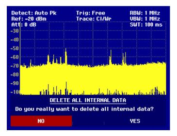
Turn the instrument off and remove the power supply unit. This will clear any data in the video- and measurement SRAM.
